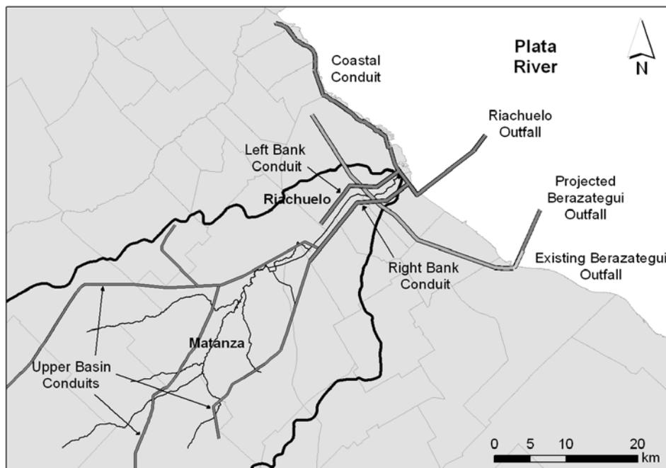
**Figure 2.** Scheme of wastewater disposal project
