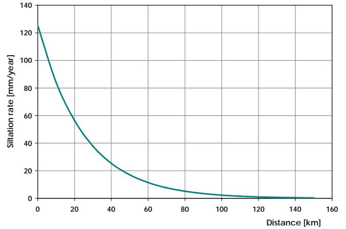
Figure 11. Distribution of siltation rate along the IPR.
