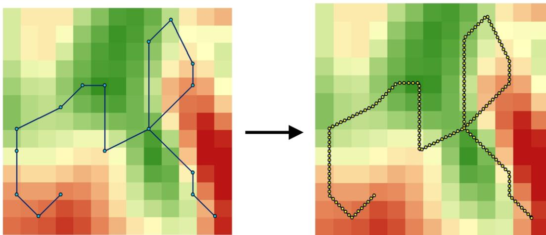
**Figure 1.** Segmentation of the pipeline route. The quadrangles indicate the elevations of the cells corresponding to the DEM.
